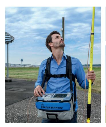
**Application example:** Bearing measurement on a terminal VOR with R&S<sup>®</sup>EVSG1000
